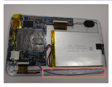
• Locate the gray cord attached to the motherboard and the battery. This is the wifi antenna.
