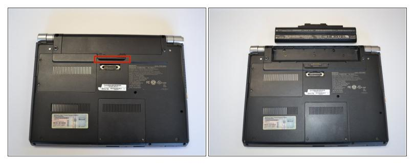
• Use a fingernail or plastic opening tool lift the battery while holding the release latch. Rotate the battery up and away from you to remove it from the laptop.
