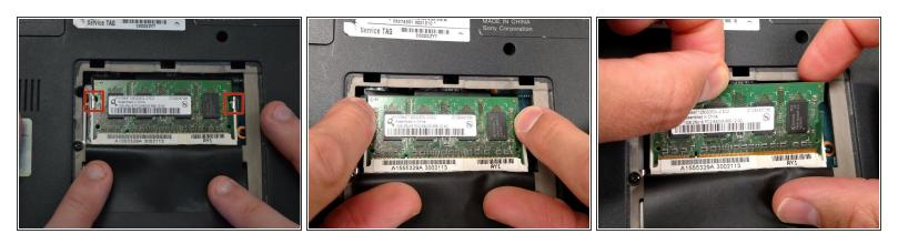
Using the same light outward pressure on the locks, lift the secondary RAM up and slide it away from you to remove it from its slot.
