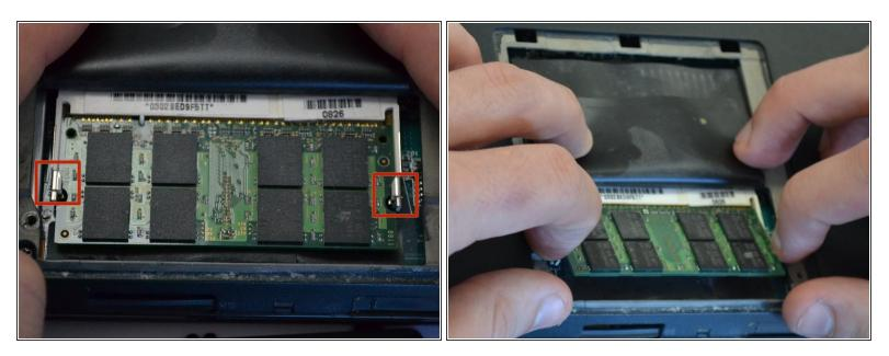
Apply light outward pressure to the locks on either side of the RAM. Rotate the RAM up slightly.
