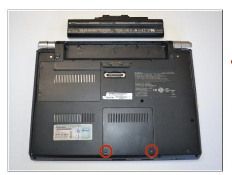
Using a Phillips #1 screwdriver, remove both screws. The screws are secured to the cover with retaining clips.
