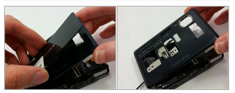
Wiggle sliding lens cover after all screws are removed and separate from front cover.
