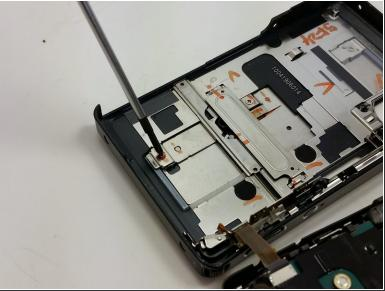
Remove the three 4mm length screws located on the inside of the front cover with the Phillips #00 screwdriver.
