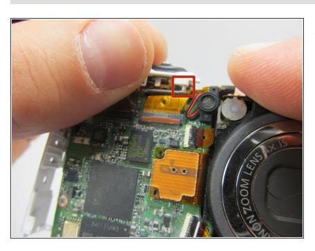
To reattach the speaker housing to the rest of the camera, make sure the pins and clips are aligned.
