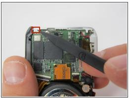
Gently remove the tabs surrounding the power button on the housing of the camera.
