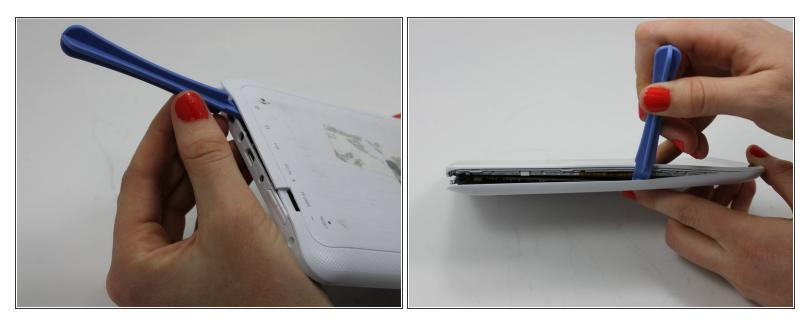
• Use the plastic opening tool to assist in removing the back cover.
