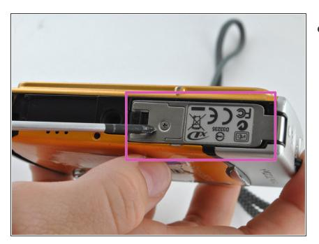
Locate the battery latch on the bottom of the device.
