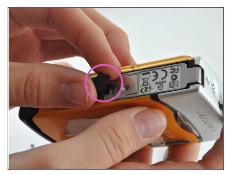
Remove the small black plastic piece positioned at the opening side of the battery latch.
