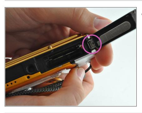
Locate the screw in the center crease of the opening of the battery latch.
