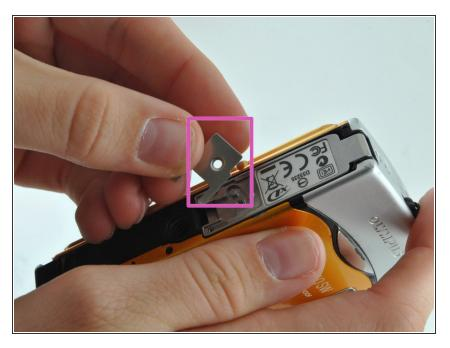
You will now be able to lift and remove the thin metal covering from battery latch.
