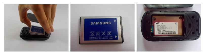
• Pop out the battery by placing your finger in between the open slit.
