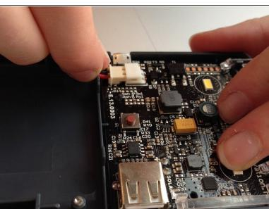
While placing the new battery, make sure the connector is not upside down as you can see in the first picture. Click it in the PCB.
