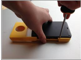
Turn the Waka Waka upside down. Make sure the Waka Waka is placed on a flat surface. Place the flathead screwdriver between the yellow and the black part as can be seen in the second picture. Force will be needed. If one side came loose, do the same for the other side.
