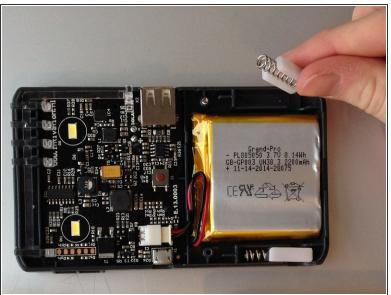
Push the electricity cables aside. Place the springs in the case next to the battery.
