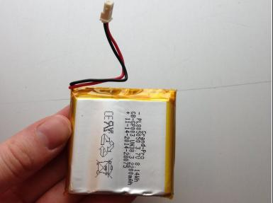
Remove the battery from the PCB by pulling the cables out of the clicking system.
