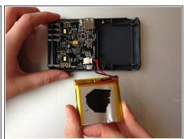
Now you see all the components in the Waka Waka. The battery is attached to the case with tape, so you have to use force to pull it off.
