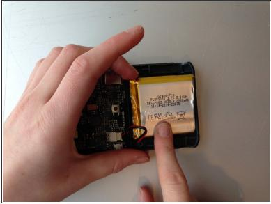
Use double sided tape to attache the battery to the case. Place the battery back in the case as shown in the second picture.
