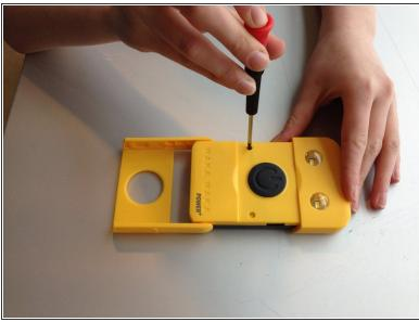
First you remove the two yellow rubbers using your nail or the screwdriver. Than use the Phillips screwdriver to remove the two screws.
