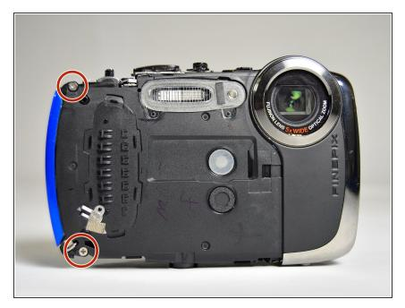
Using Phillips #00 screwdriver, remove the two 3.0 mm screws.
