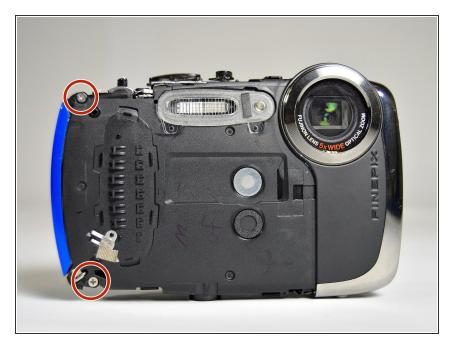
Using Phillips #00 screwdriver, remove the two 3.0 mm screws.
