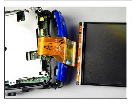
Detach the LCD screen from the motherboard by detaching the orange ribbon. To reassemble your device, follow these instructions in reverse order.
