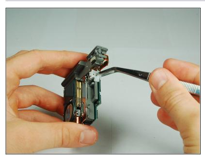
Use <u>tweezers</u> to remove the small white piece from the motherboard assembly.
