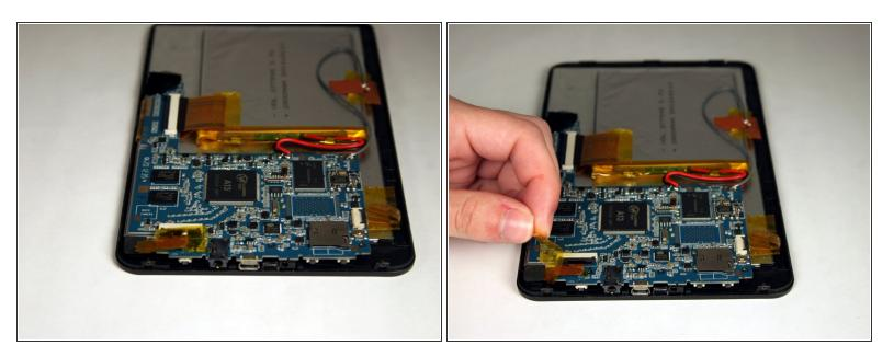
Once the panels are separated, remove the tape holding down the ribbon connector that is connecting the camera to the motherboard.
