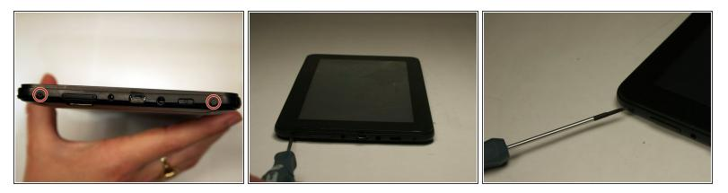
Unscrew the two (2) 1.3mm Phillips #00 screws found on the bottom edge of the tablet, where the power and volume buttons are located.
