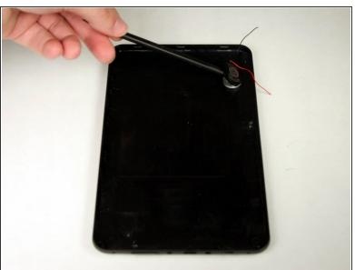
Insert the flat end of the spudger between the casing and the speaker. Push inwards to pry the speaker from the casing.
