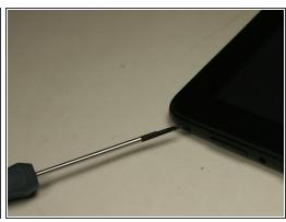
Unscrew the two (2) 1.3mm Phillips #00 screws found on the bottom edge of the tablet, where the power and volume buttons are located.
