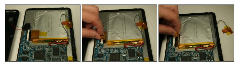
• Lift up the two pieces of tape holding the copper plate and the connector ribbon to the battery. Gently hold or place away from the battery.
