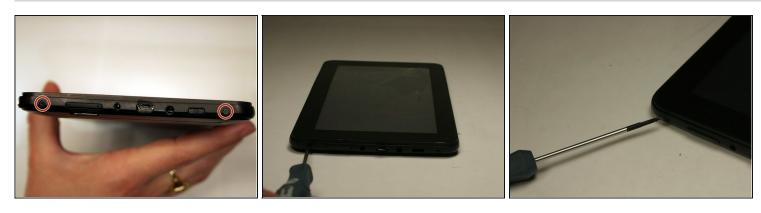
Unscrew the two (2) 1.3mm Phillips #00 screws found on the bottom edge of the tablet, where the power and volume buttons are located.
