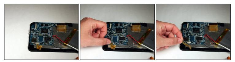
• Rotate the tablet 180 degrees and flip up the black lever of the connector holding the small, yellow ribbon. Remove ribbon from the connector.
