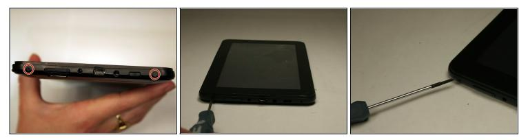
• Unscrew the two (2) 1.3mm Phillips #00 screws found on the bottom edge of the tablet, where the power and volume buttons are located.
