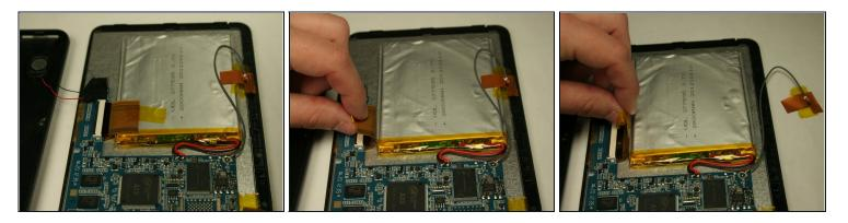
• Lift up the two pieces of tape holding the copper plate and the connector ribbon to the battery. Gently hold or place away from the battery.
