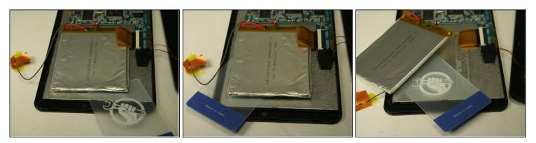
• Using a <u>plastic card</u>, gently break the adhesive that holds the battery to the metal screen plate.
