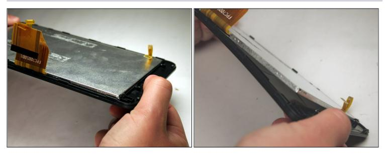
• Once the battery and motherboard have been removed, gently bend the screen plate to pop out the metal digitizer that sits on the glass and plastic screen.
