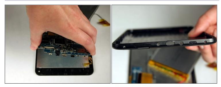
• With the motherboard detached from the screen plate, there is now access to the electrical components under the motherboard and the mechanical button components on the back plate.
