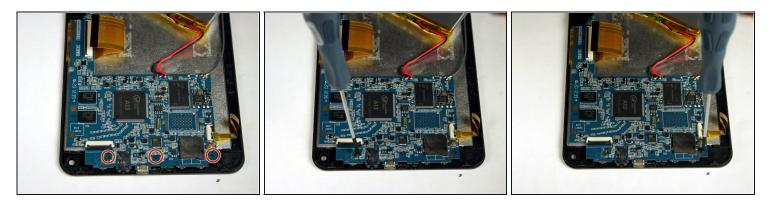
• Rotate the tablet 90 degrees and remove the three (3) 1.3 mm Phillips #00 screws that hold the motherboard in place.
