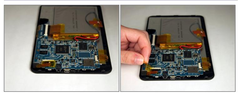
• Once the panels are separated, remove the tape holding down the ribbon connector that is connecting the camera to the motherboard.
