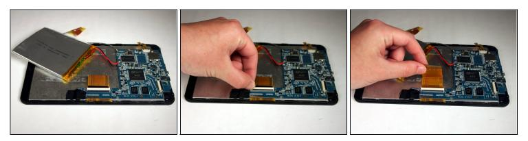
• Once battery is removed, flip up the black lever of the connector that is holding the wide ribbon in place for the screen. Remove the ribbon from the connector.
