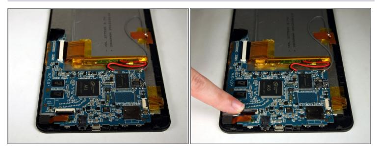
• Lift up the black lever of the connector that holds the camera ribbon in place.
