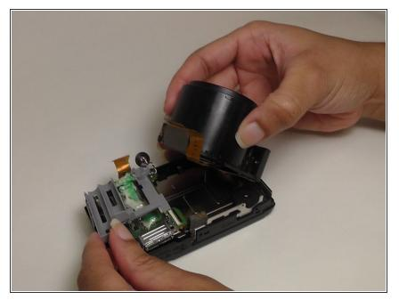
• Lift the lens and attached ribbon cables from the camera in order to switch this lens with a new one.
