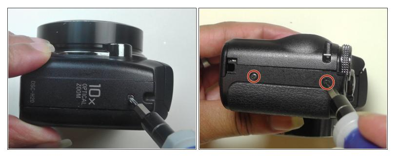
• Remove the screws on the left and right sides of the camera.
