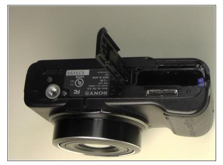
Place the camera upside down with the battery port positioned upward and the battery port open.
