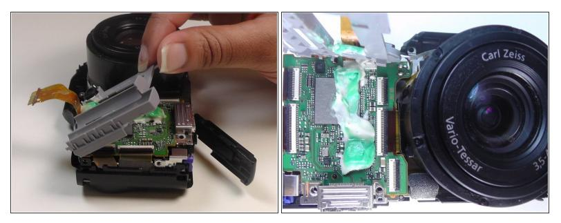
• Lift up the gray plastic facing in order to uncover the motherboard and the ribbon cable ports.
