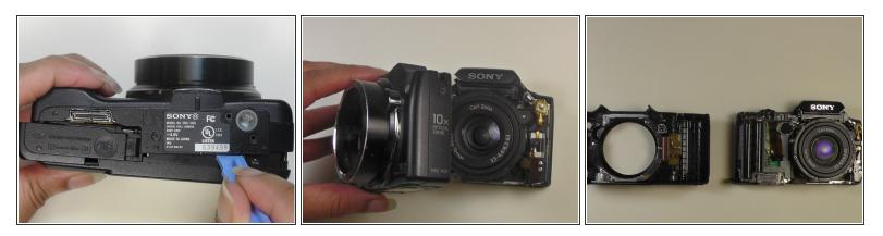
• Pry the front cover of the camera off with the plastic opening tool.
