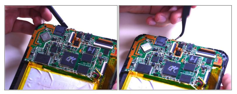
• Gently lift the motherboard up to extract the charging port out with the tweezers.
