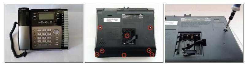
Remove the eight 11mm screws found on the bottom side of the base with a Phillips #00 screwdriver.
