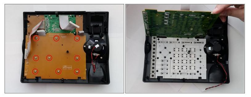
Remove the nine 11mm screws from the board using a Phillips #00 screwdriver, in order to expose the keyboard pressure sensors.
