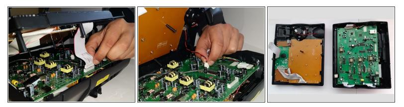
• Unclip the wires that connect the front piece to the circuit board on the back piece.
