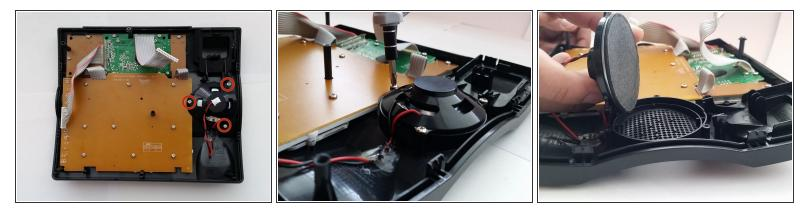
Use a Phillips #00 screwdriver to remove the three 11mm screws to separate the speaker from its base.
