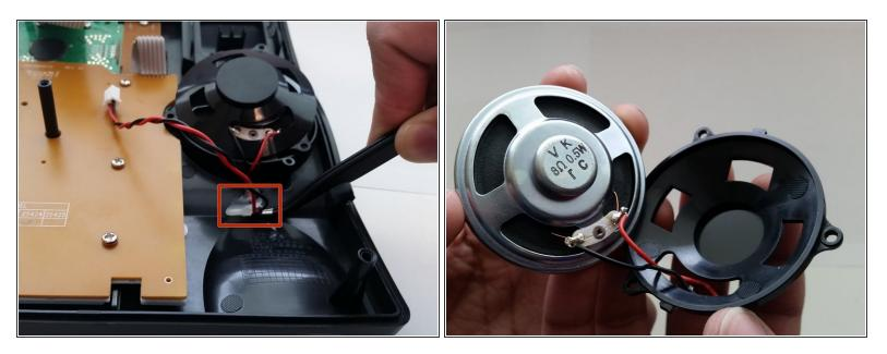
• Once the screws are taken out, use tweezers to remove the hot glue from the wires.
