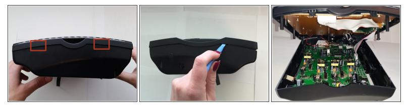
• Use a plastic opening tool to separate the back and front pieces.
