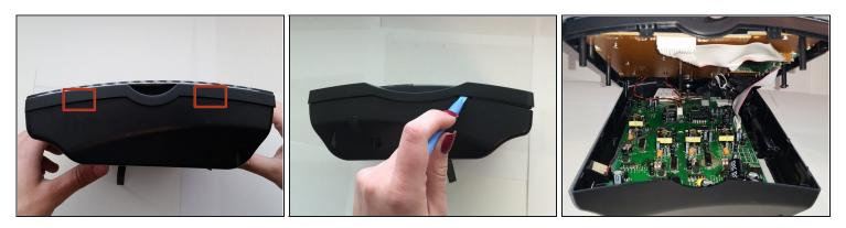
Use a plastic opening tool to separate the back and front pieces.
