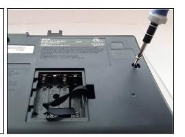
Remove the eight 11mm screws found on the bottom side of the base with a Phillips #00 screwdriver.
