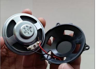
• Once the screws are taken out, use <u>tweezers</u> to remove the hot glue from the wires.
