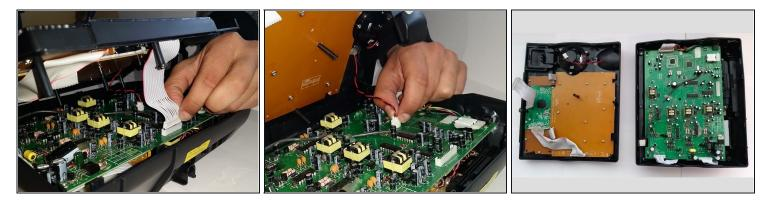
• Unclip the wires that connect the front piece to the circuit board on the back piece.
