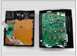
Unclip the wires that connect the front piece to the circuit board on the back piece.
