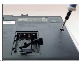
Remove the eight 11mm screws found on the bottom side of the base with a Phillips #00 screwdriver.
