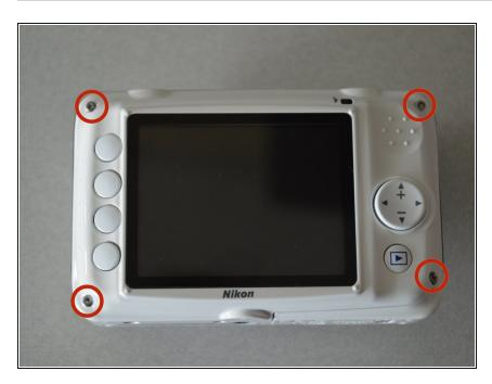
Remove the four screws the hold the back of the case to the rest of the camera.
