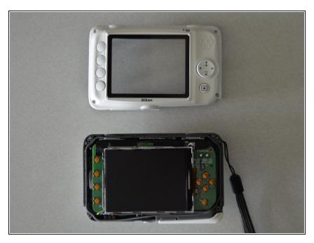
Remove back case from the rest of the camera carefully.
