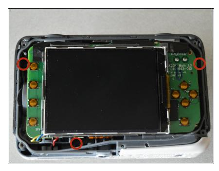
• Remove the three screws the secure the motherboard to the front case.
