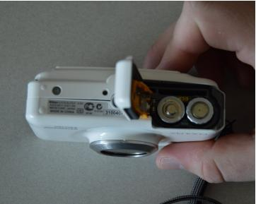
Slide the second cover (yellow) to the right (similar to the outer cover). This will allow the batteries to be exposed.
