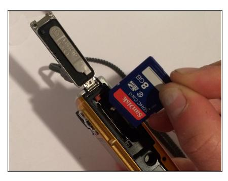
Hold the memory card so that the pointed wedge is facing up and the sticker is facing the front of the camera.
