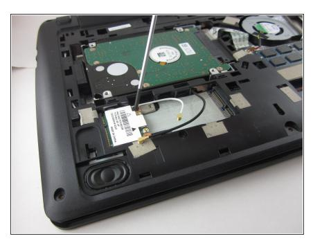
Remove the 4mm Phillips #1 screw holding the WLAN card holding it in place.
