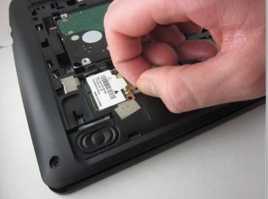
Unplug the white and black cables connecting the WLAN card.
