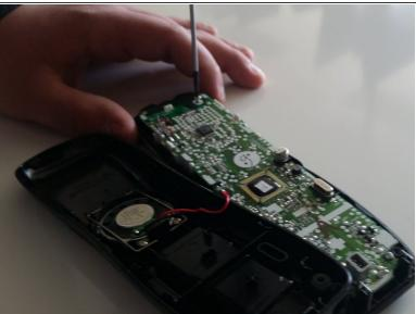
Carefully remove the 9mm Phillips #1 screw from the top corner of the circuit board.
