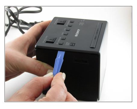
Using the opening tool, gently pry the top portion from the side section of your device.
