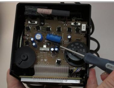
• Using the Phillips #00 screwdriver, remove the two 14mm screws from the top of the motherboard.
