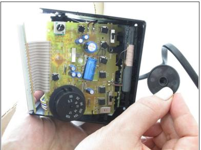
Remove the volume dial by pulling it off the motherboard. This can take a little force to remove.
