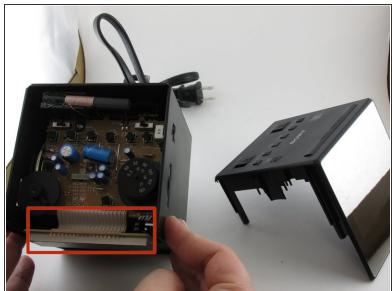
Carefully separate the device by gently pulling up on the top of the clock/radio.
