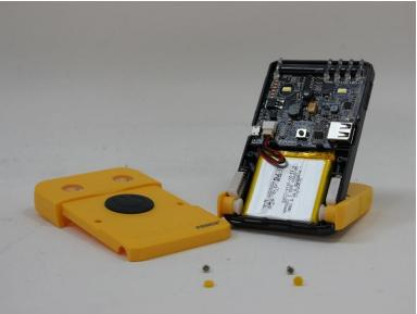
⚠ Be careful not to damage the plastic during this step! Using a plastic opening tool instead of a screwdriver may be advisable.
