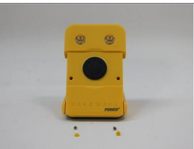
Open the lid, remove the silicone screw covers and undo the screws.
