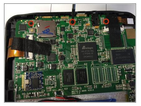
There are 3 Ph 00 screws (4 mm long) that connect the motherboard to the tablet. These screws are indicated in the image by special markers. Once you have located these screws, unscrew them.
