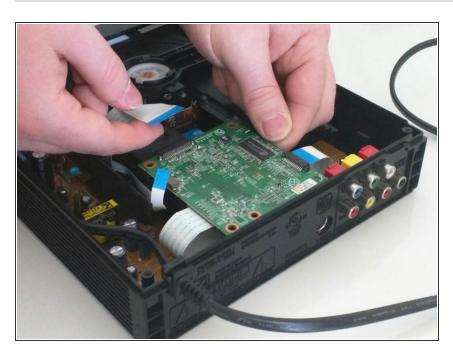
Unplug wires from motherboard component. Do not be afraid to tug.
