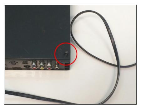
Remove two screws on top panel.
