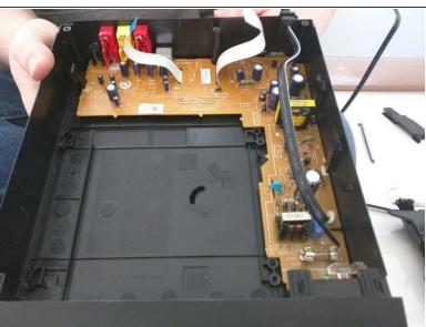
Remove disc drive by unscrewing the 2 screws that hold the drive in place.
