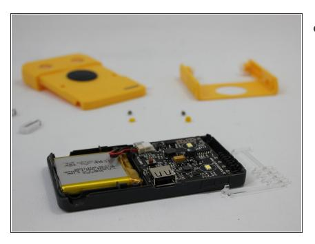
This can simply be pulled out once the covers are removed.
