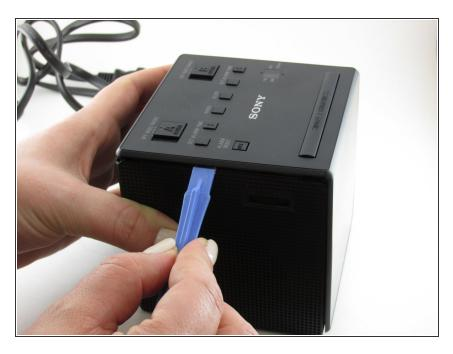
Insert the plastic opening tool to pry apart the top and sides of the device gently.
