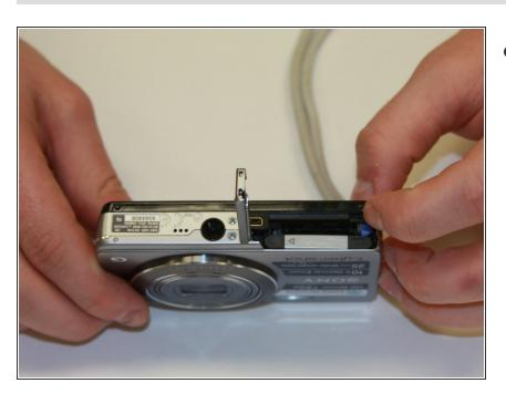
Open the battery lock to release the battery.
