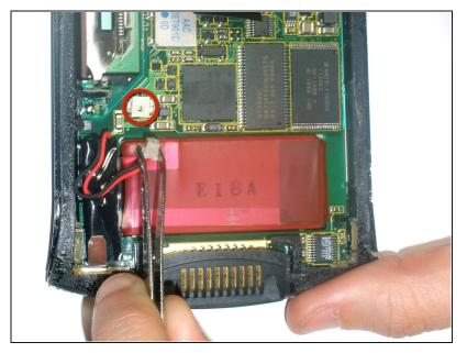
Using the <u>tweezers</u>, carefully disconnect the battery cable from the port
