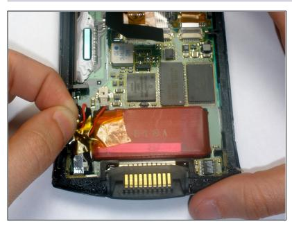
Remove the yellow tape that is covering the battery connector
