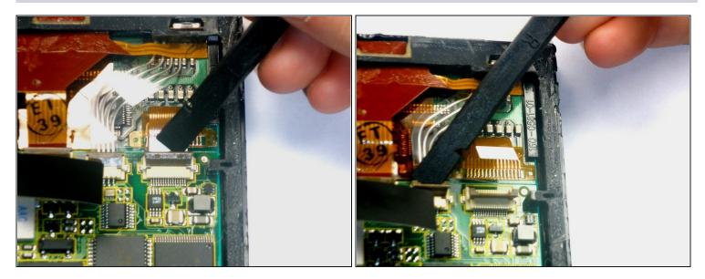
• Using the spudger lift the tabs holding the LCD/Digitizer combo cables to the WorkPad.
