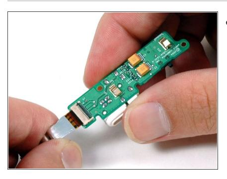
Pull the orange headphone jack cable directly out of its connector.
