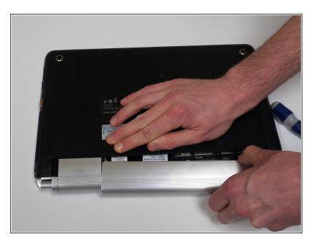
Remove battery by sliding the battery ejection switch to the right and pulling the battery away from the laptop.
