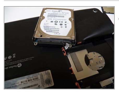
Remove old hard drive from its slot and replace with new hard drive, sticker side facing up. To reassemble your device, follow these instructions in reverse order.
