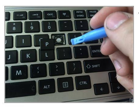
Take the tool and pry the designated key completely off of the keyboard.
