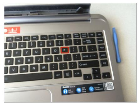
First, identify which key(s) need to be replaced, and make sure a replacement key is purchased, i.e. the 'p' key.
