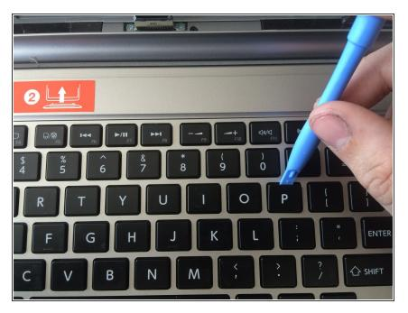
Take the plastic opening tool and wedge it under the key you are replacing.
