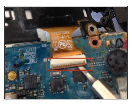
With the flathead, lift up cable lock and pull the film out from underneath the lock.
