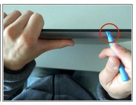
Take the pry tool and pry open the backing of the tablet around all four sides and pull off back.
