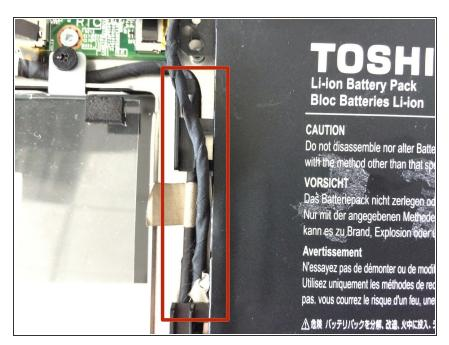
Remove shown wires from clips on the left hand side of the battery before pulling the battery completely out.
