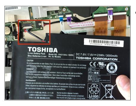
Remove highlighted plug out of the circuit board before completely removing the battery pack.
