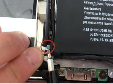
Use a Phillips #0 Screwdriver to remove four screws in the corners of the battery pack.
