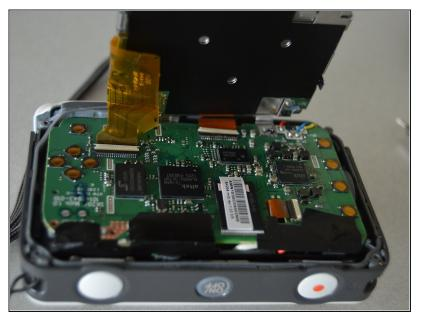
Spin the camera around and gently pull the screen towards you. This will allow easy access to components on the motherboard.
