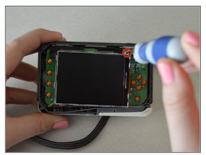
Remove screw connecting the top right of the screen to the mother board.
