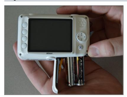
Remove the batteries by gently tipping the camera.
