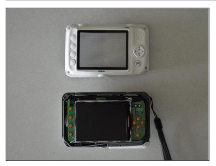
• Gently separate the back panel from the rest of the camera.
