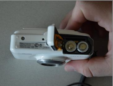
• Slide the second cover (yellow) to the right (similar to the outer cover). This will allow the batteries to be exposed.
