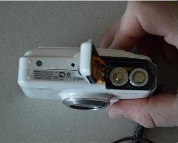
Slide the second cover (yellow) to the right (similar to the outer cover). This will allow the batteries to be exposed.
