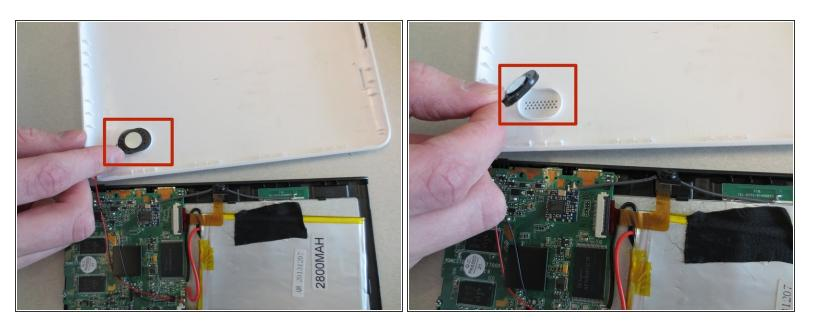
• To completely remove the base from the top of the tablet, peel the microphone from the back.
