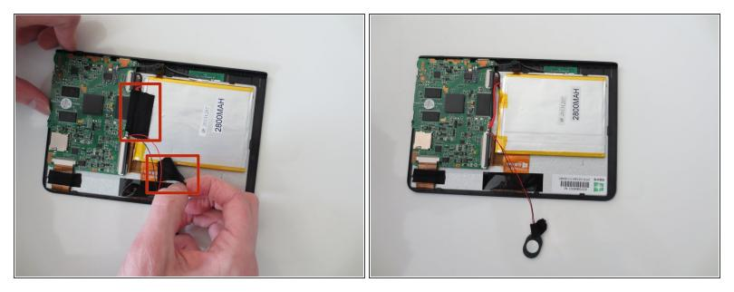
• Remove the two pieces of tape holding the battery in place by gently peeling it off.
