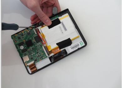
• Use your 00 phillips head screwdriver to remove the three 4mm phillips screws circled in red.
