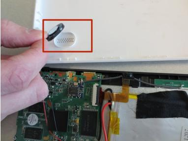
Peel the microphone from the back of the device.
