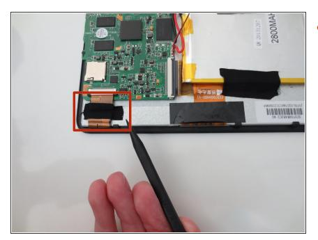
Remove the tape from the indicated copper strip.
