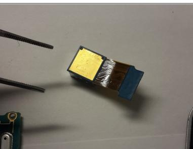
Use a pair of pliers to remove the rear facing camera
