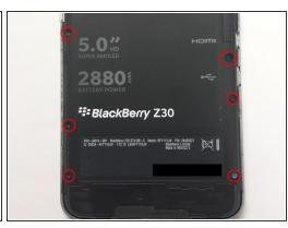
Locate and unscrew all 10 T5 screws around the back cover
