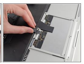
• Use the tip of a spudger or your fingernail to flip up the retaining flap on the trackpad ribbon cable ZIF socket.
