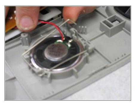
Release the speaker from the locking pin by pushing down on each ending side of the pin and pushing it away from the speaker.
