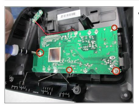
Unscrew bottom shell circuit board screws(Head size: 4mm Length: 8.6mm).
