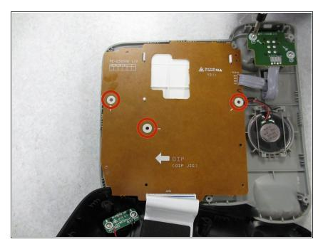
Unscrew the 3 screws(Head Size: 4mm Length: 8.6 mm) from the top shell circuit board.
