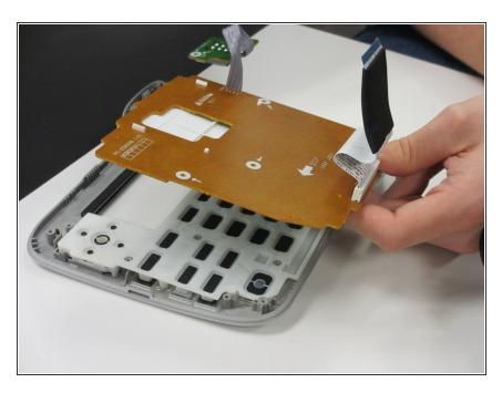
Remove top shell circuit board by lifting the circuit board out of the case
