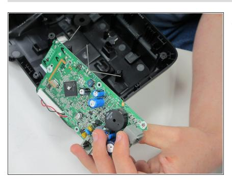
Lift bottom circuit board from the bottom shell.
