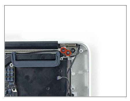
Remove the two 4.9 mm T8 Torx screws securing the antenna cable retainer on the left display hinge to the upper case.
