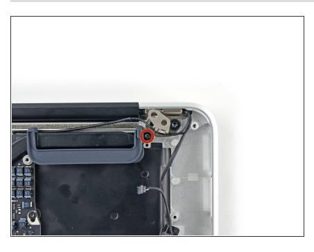
Push the antenna cable retainer out of the way and remove the single 3 mm T5 Torx screw securing the end of the heat sink to the upper case.
