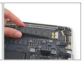
Lift the free end of the SSD up slightly and pull the SSD straight out of its socket on the logic board.
