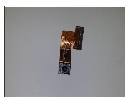
Once the cable is removed from the motherboard, the entire camera can simply be removed from the device.
